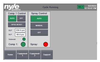
**Comp 1 Control:** allows you to control the compressor as well as monitor the line pressures.
