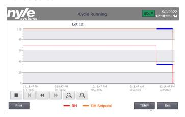
7. If there is an issue with the unit, an alarm indicator will pop up on the top right column of the home screen. You can select this to view the alarm screen.
