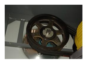
The belt tension must be correct. If too tight, reduced bearing and belt life will result. If too loose, belt life will be shortened due to slippage. The ideal situation would be for the belts to be as loose as possible without squealing.
